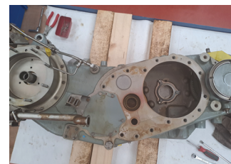
No. 2 Spur Gear Removed
