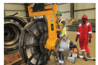
LM2500+G4 HPT Assembly Removal
